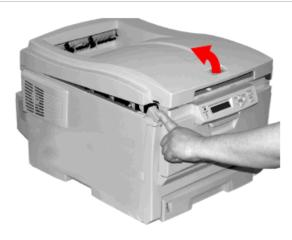
2. Pull the two blue fuser lock levers (1) towards the front of the printer.
